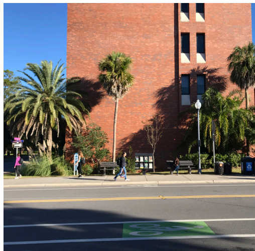
The planting and furnishings zone along Buckman Drive; The lack of a defined furnishings zone along Stadium Road
