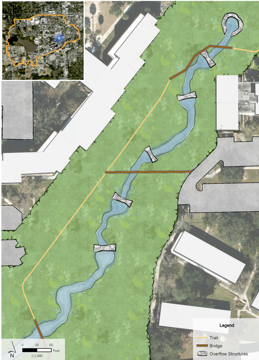
Figure 9. Jennings Creek Headwall and Step-Pool Improvements
