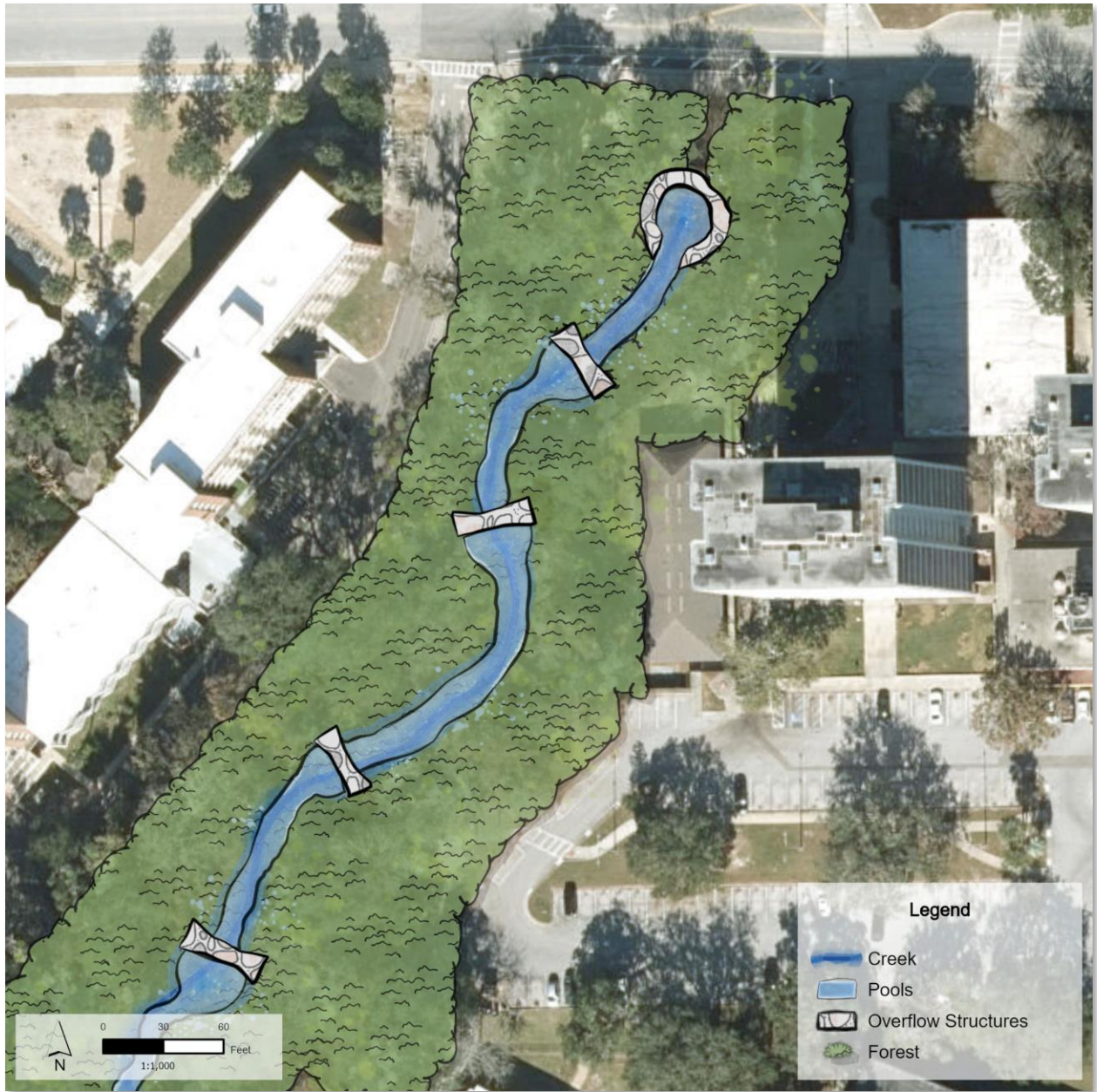
Figure 10. Jennings Creek Step-Pool Stabilization Concept
