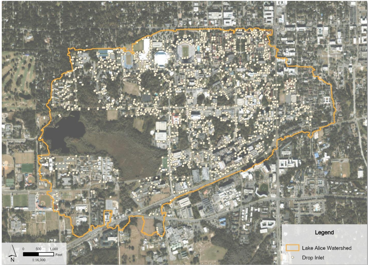
Figure 3. UF Stormwater Drainage Structures within the Lake Alice Watershed (2023)
