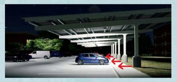
The vertical structural columns supporting the canopy will actually be installed along the left (West) edge of the sidewalk, not in the grass area as shown in these renderings.
